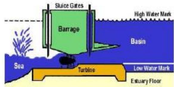
**Fig.2:** Tidal barrage
