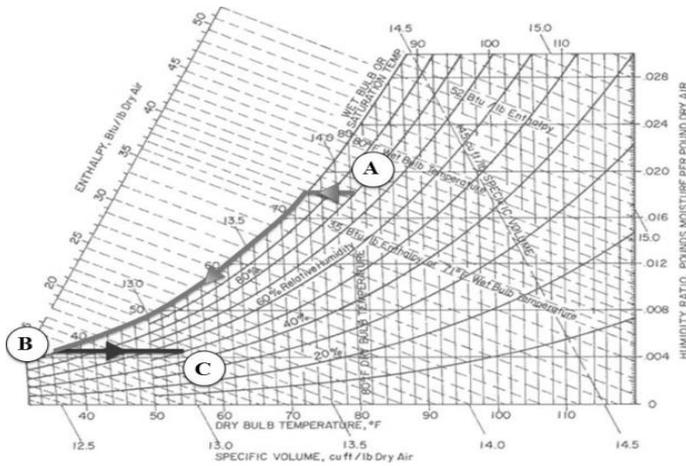
**Fig.14** Conventional Cooling and Dehumidification Process in Psychrometric Chart
