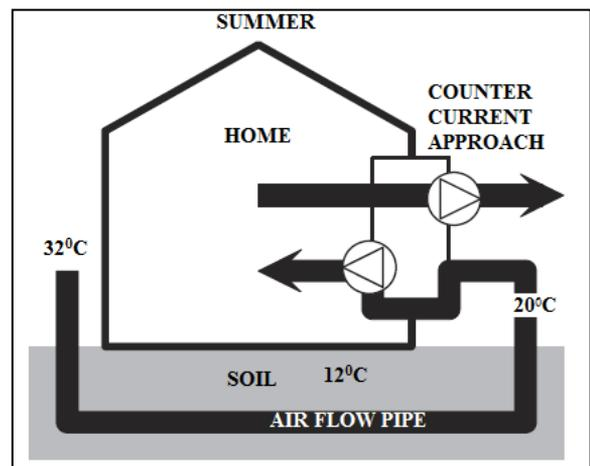
**Fig.9** Experimental Configuration by Pierre et al [12]
