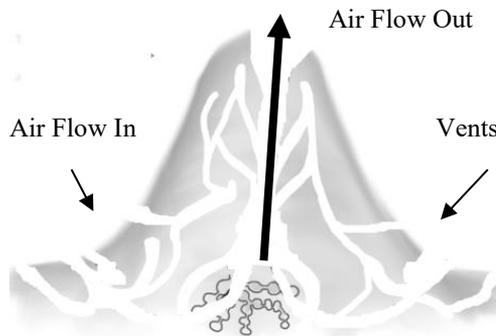
Fig.3 Air Flow in a Termite Mound (Open Mound)
