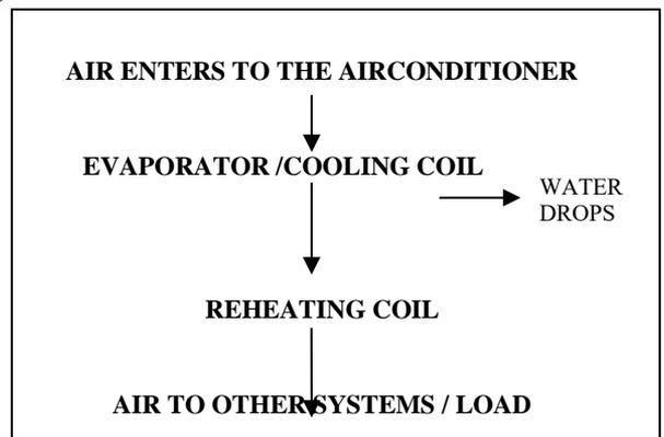
**Fig.13** Scheme in Conventional Air Conditioners
