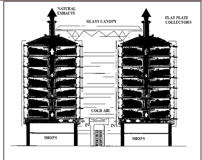
Fig.5 Ventilation at East Gate Center, Harare
