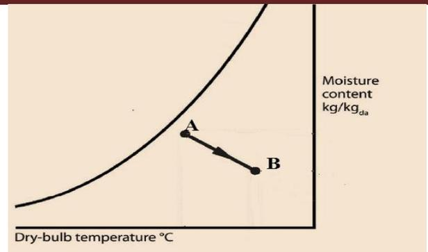
**Fig.15** Desiccant based Dehumidification
