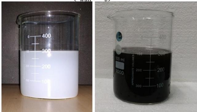
Fig. 3: Al<sub>2</sub>O<sub>3</sub>-water and CuO-water nano-fluid (0.05%) [3]
