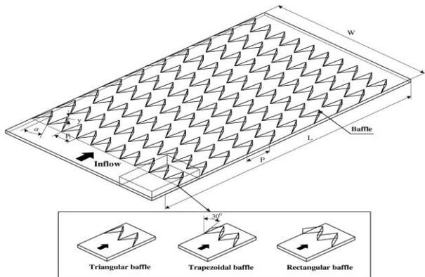
**Fig4:** Test section with rectangular, triangular, and trapezoidal baffles.
