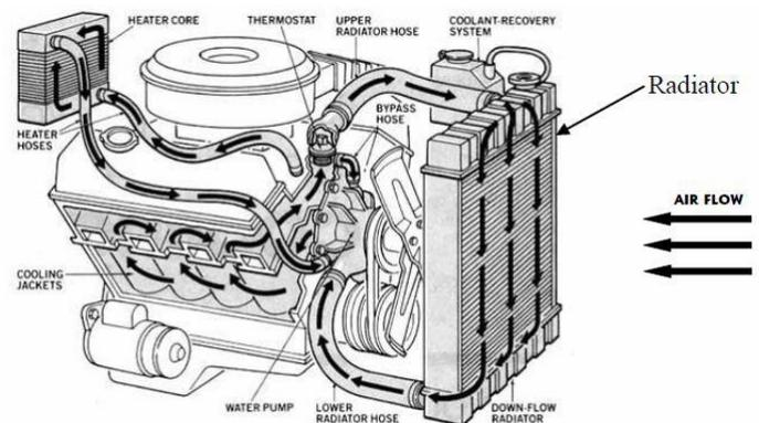
Fig.1: Schematic of Radiator [3]
