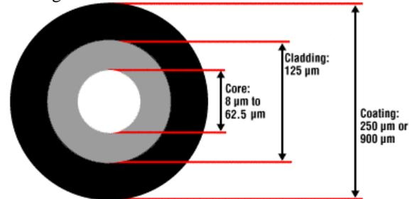
Fig: 3.5. Cross section of a typical fiber
