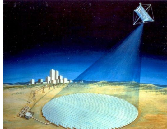
Fig. 4. Rectenna- power is beamed to a receiving antenna or “rectenna” on Earth [4]
