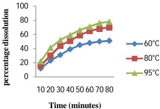
**Fig. 1.** Percentage dissolution of iron against time
