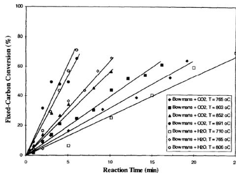
**Fig. 4.** Fractional conversion versus reaction time for CO<sub>2</sub> and H<sub>2</sub>O gasification of Bowmans coal at different temperatures [14].
