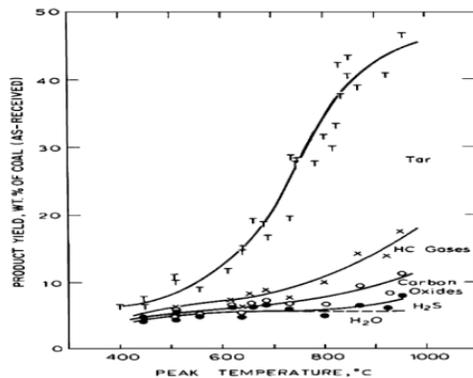
**Fig. 1.** Yield of pyrolysis products increases as peak temperature increases [10].
