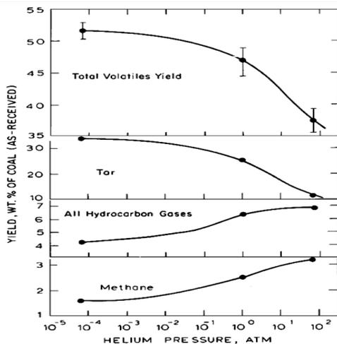
**Fig. 3.** yield of products verses pressure during pyrolysis (Pittsburgh no. 8 coal at 997oC)[10].
