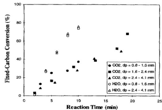
**Fig. 5.** Fixed carbon conversion of Bowmans coal during H<sub>2</sub>O and CO<sub>2</sub> gasification for different particle size at reaction temperature of 765°C [14].
