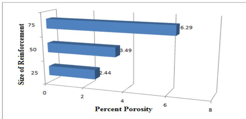
**Fig: 3.** Percentage Porosity of AA6082/SiC metal matrix composite
