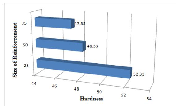
**Fig. 5.** Hardness of AA6082/SiC metal matrix composite
