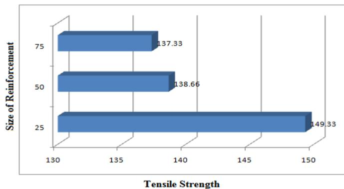
**Fig. 4.** Tensile strength of AA6082/SiC metal matrix composite
