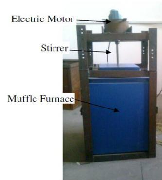
**Fig: 1.** Experimental Set-up of Mechanical Stir Casting Process
