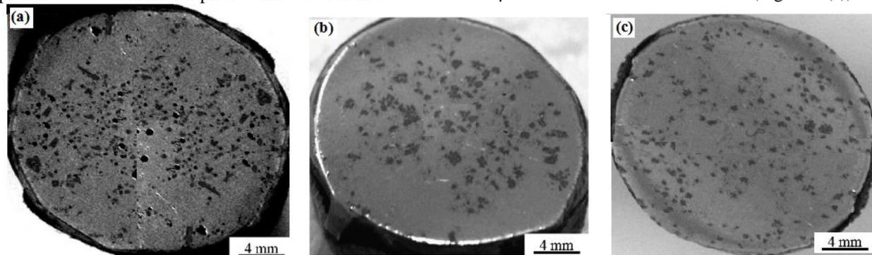
**Fig: 2.** Macrostructure of AA6082/SiC MMC: (a) 75 µm of SiC, (b) 50µm of SiC, (c) 25 µm of SiC
