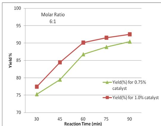
Fig. 2. Time v/s Yield (%) for molar ratio 6:1 and different catalyst percentage
