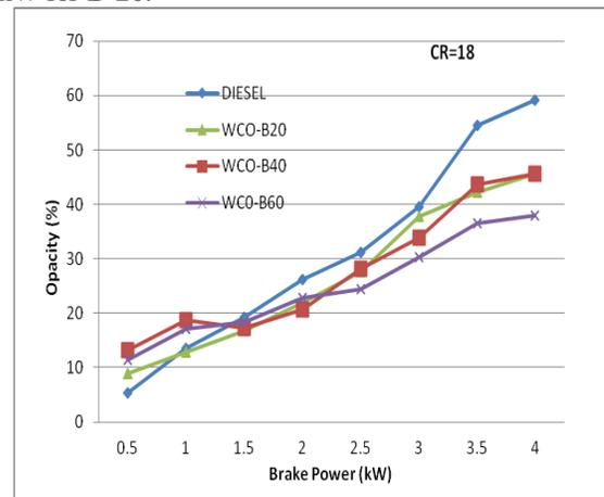
**Fig. 7.** Comparison of smoke opacity v/s brake power
