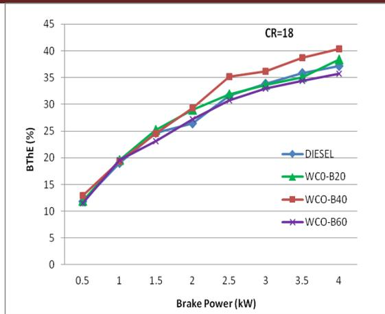
**Fig. 4.** Comparison of brake thermal efficiency v/s brake power
