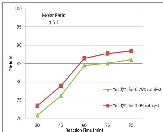
Fig. 3. Time v/s Yield (%) for molar ratio 4.5:1 and different catalyst percentage
