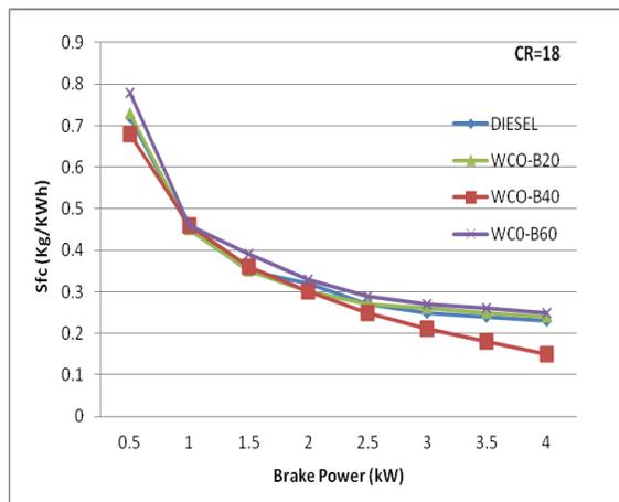
**Fig. 5.** Comparison of specific fuel consumption v/s brake power
