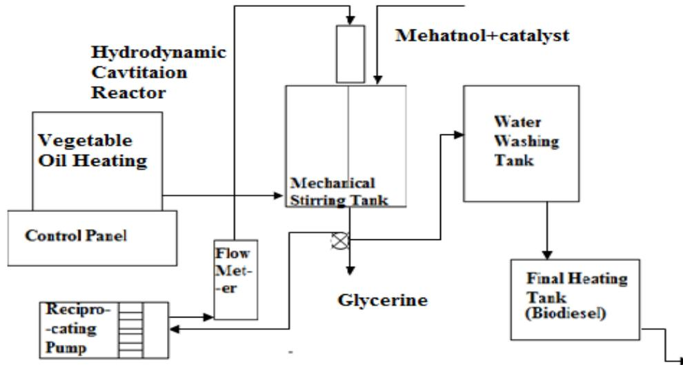
Fig. 1. Schematic representation of biodiesel reactor
