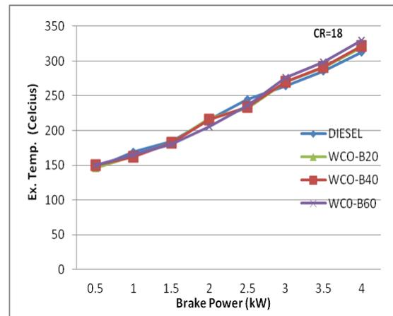
**Fig. 6.** Comparison of exhaust gas temperature v/s brake power
