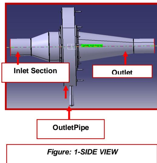
Venturimeter to ensure smooth flow of air through the shutter.
