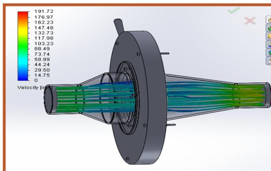
possible permutations and combinations in these values, we have carried out analyses on proposed 5 leaf iris shutter, and the design passed in all the flow analyses carried out.
