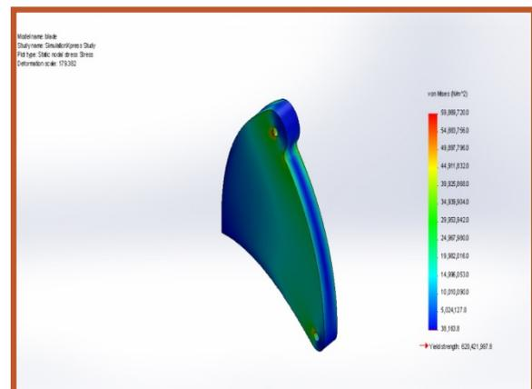
Fig. 3. Stress Analysis on Blade at 3.7 bar
