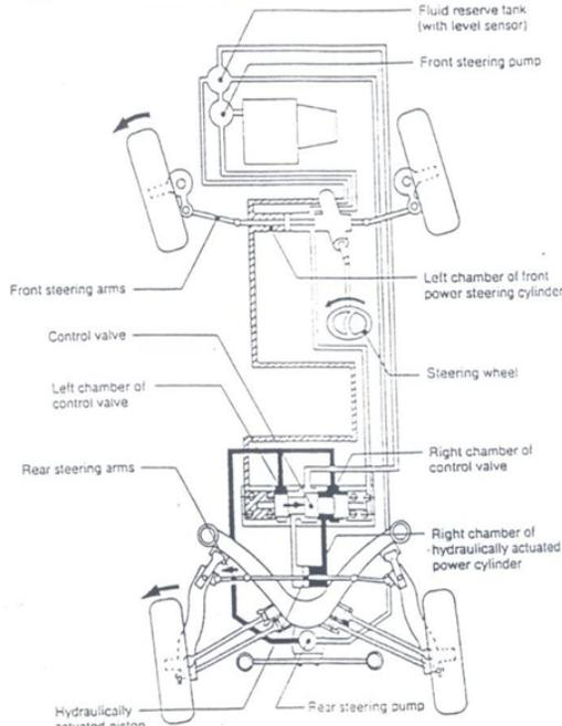
**Fig: 5.** 4 Wheel Steering mechanisms
