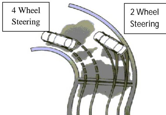
Fig 2: Comparison between two drives
