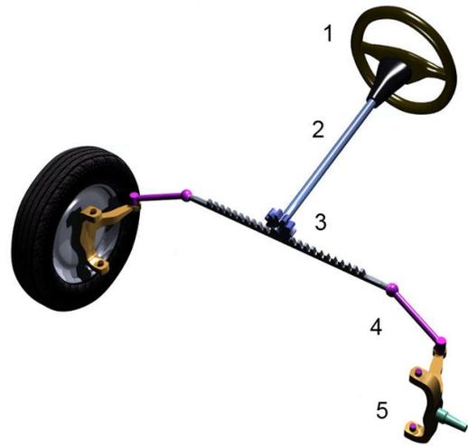
**Fig: 1.** Rack and pinion steering mechanism
