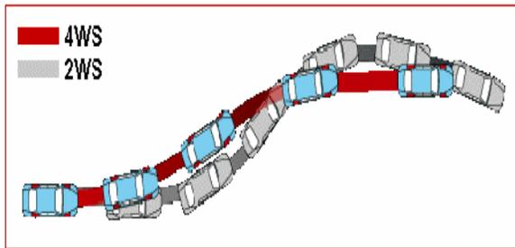
**Fig: 3.** Comparing turning radius for a 4WS and a 2WS
