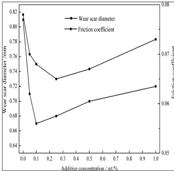
**Fig. 2.** Wear scar diameter and friction coefficient as a function of surface-modified nano-Y<sub>2</sub>O<sub>3</sub> concentration [27]
