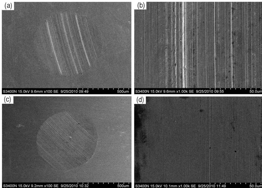
**Fig. 3.** SEM images of wear scar of the steel balls lubricated by liquid paraffin (a, b) and liquid paraffin containing surface-modified nano-Y<sub>2</sub>O<sub>3</sub> (c, d). [27]
