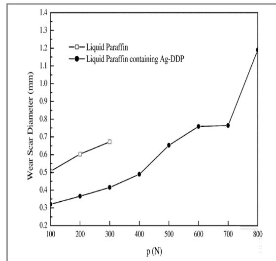
**Fig. 1.** Wear scar diameter curves of liquid paraffin and liquid paraffin containing DDP coated Ag nanoparticles with applied load [17]
