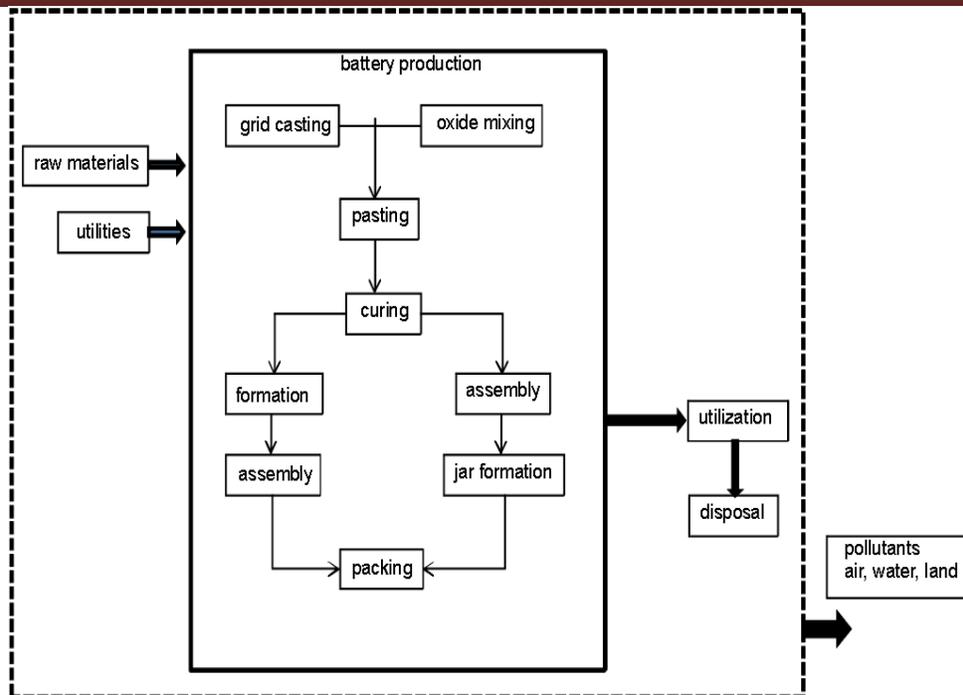
Fig. 3. System boundaries of the battery
