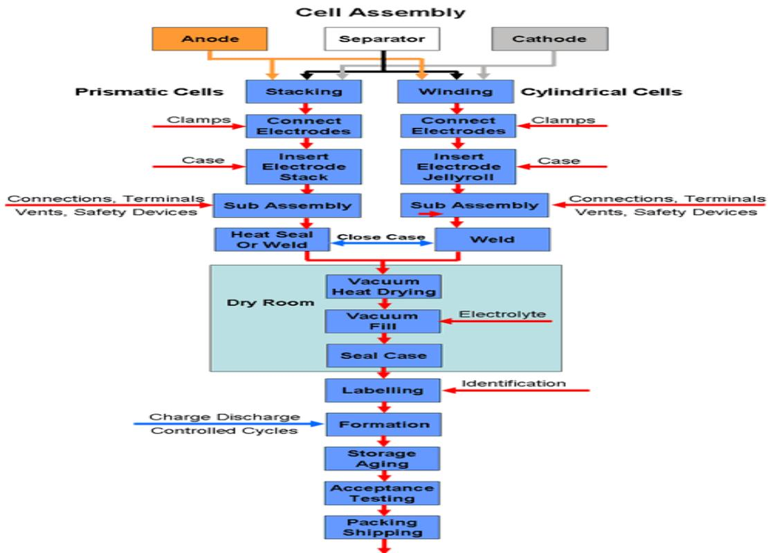
Fig: 2. Cell Assembly of a lithium ion battery
