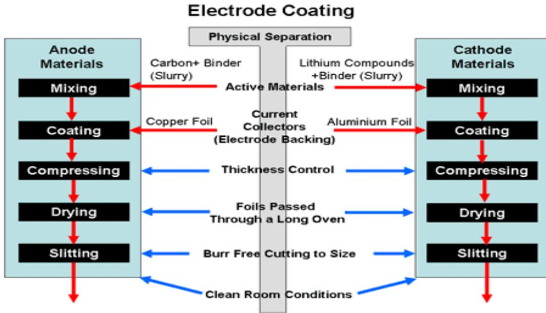
Fig: 1. Electrode coating of lithium ion battery
