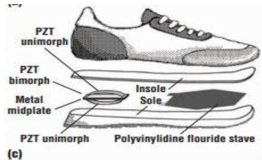
**Fig. 3.** Prototype PVDF bimorph generator for a shoe insole. Power is generated through the mechanical bending of the sole. Photos courtesy SRI, International
