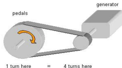
**Fig. 1.** Belt drive transmitting torque from pedal to generator. Photo courtesy
