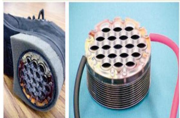
**Fig. 4.** An electrostatic generator based on compression of a charged dielectric elastomer during heel strike. Prototype implementation in a boot (left) and close-up of the generator (right), showing bellows on bottom and retaining frame on top. Photos courtesy SRI, International
