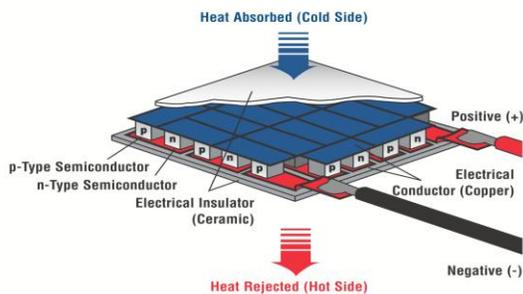
Fig: 5. A Cutaway of Thermoelectric Module
