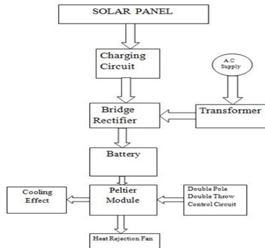
Fig. 3. Block diagram of the solar AC
