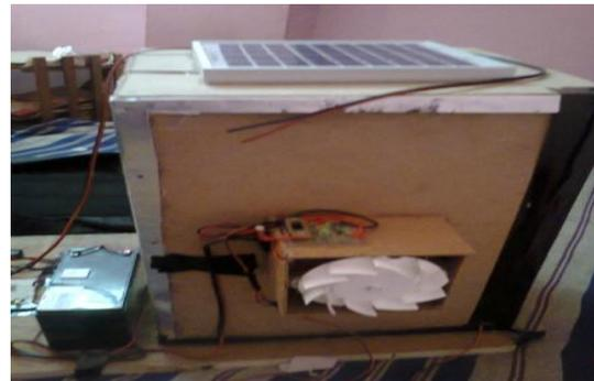
Fig: 4. Working model of A Compressor less solar AC
