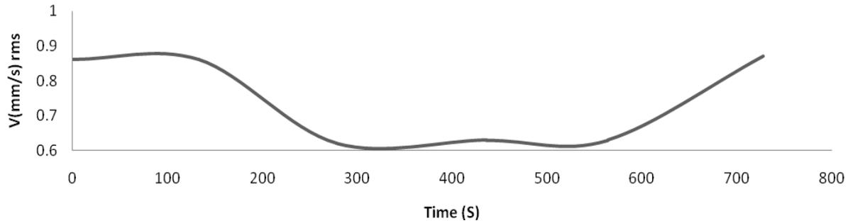
**Fig. 4.** Overall vibrations of the free end bearing in bad bearing position with ball defect
