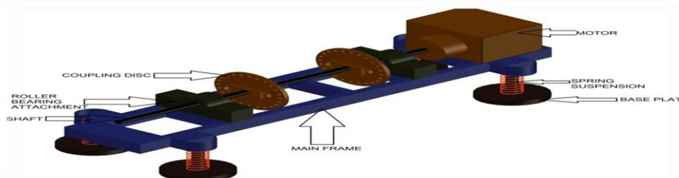
**Fig: 1.** CAD model of experimental setup. A vibration analyzer is attached on the roller bearing attachment on the free end of the rotating shaft
