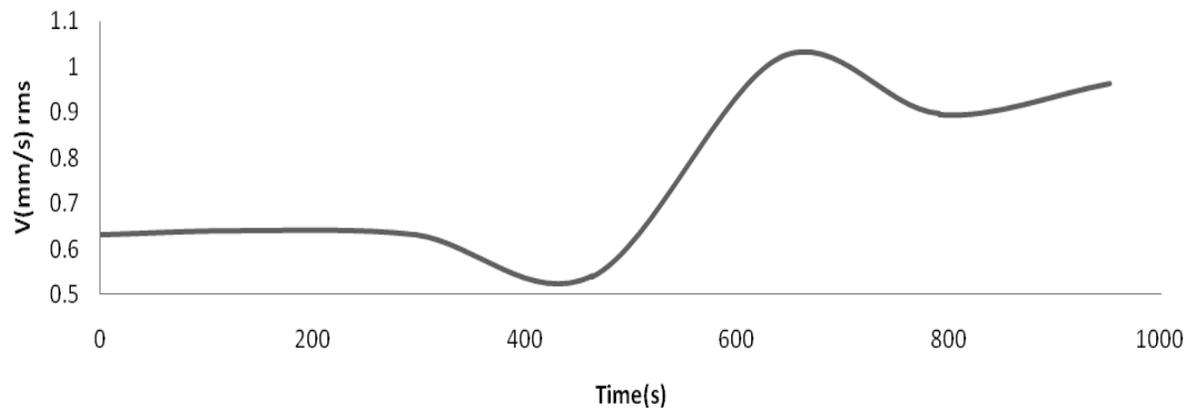
**Fig: 3.** Overall vibration of the free end bearing in bad bearing position with Outer Race defect
