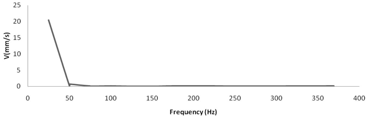
**Fig: 7.** Peak value of velocity in a bearing with Outer-Race Defect
