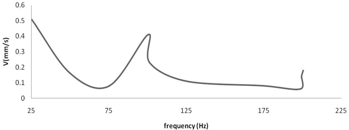
**Fig. 5.** Peak values of velocity in a Bearing with Ball Defect
