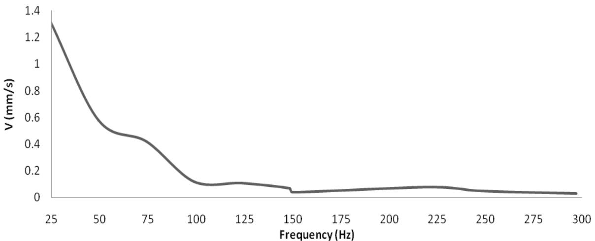
**Fig. 6.** Peak values of velocity in a Defect-Free Bearing
