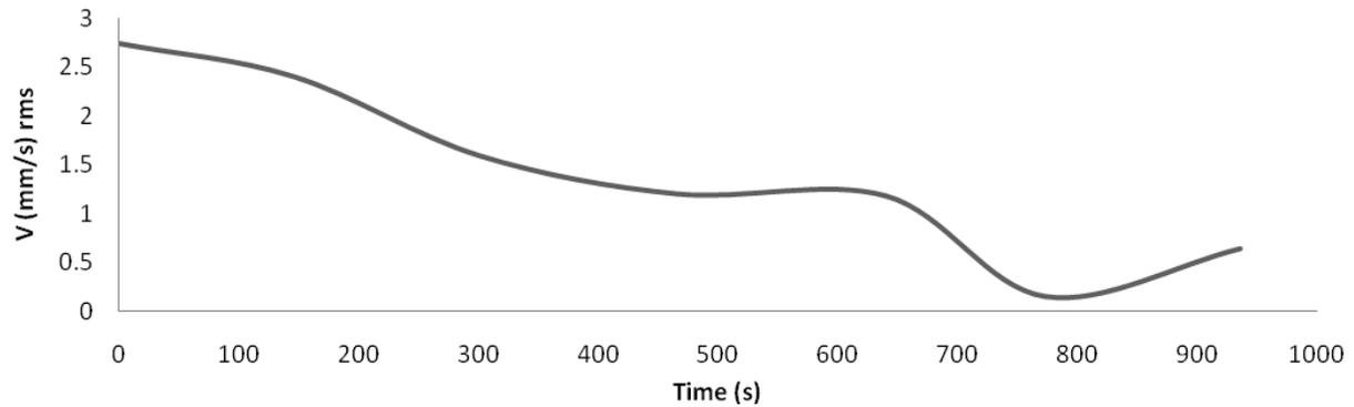
**Fig: 2.** Overall vibrations of the free end bearing in good bearing position
