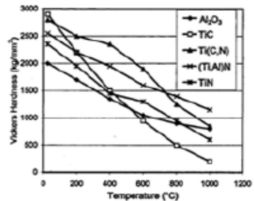
Fig. 6. Temperature dependence of micro hardness
