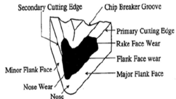
**Fig: 5.** Typical wear pattern and pertinent technology
