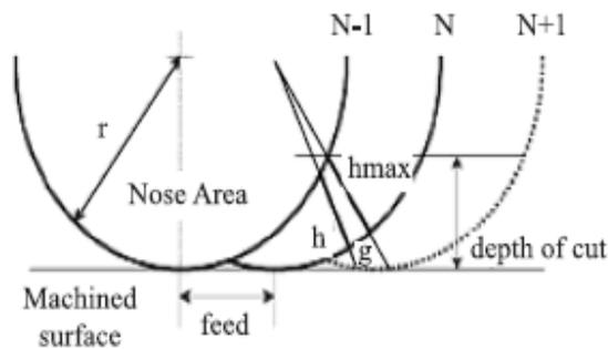
**Fig: 4.** Tool nose area showing uncut chip thickness (h) and the distance (g) from the cutting edge to the final machined surface
