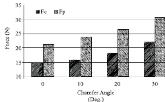
**Fig. 3.** Correlation of cutting force and chamfer angle
