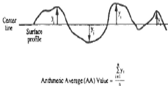
**Fig: 7.** Illustration of surface roughness
