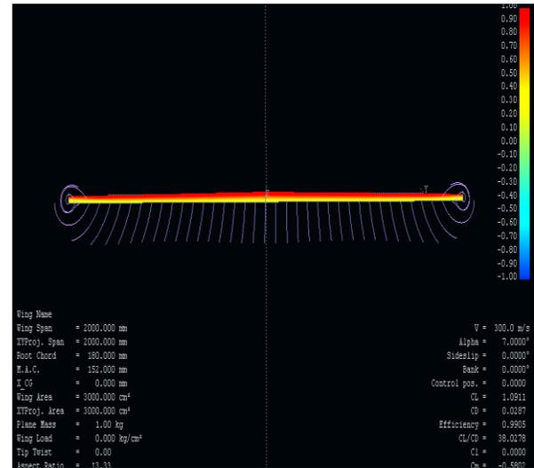
Fig: 4 (a). Vortex formation at normal wings
