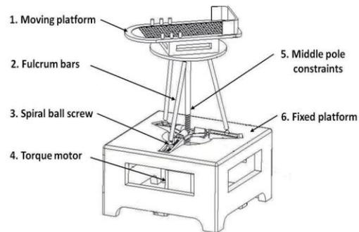
**Fig. 6.** Parallel ankle rehabilitation robot [13]
