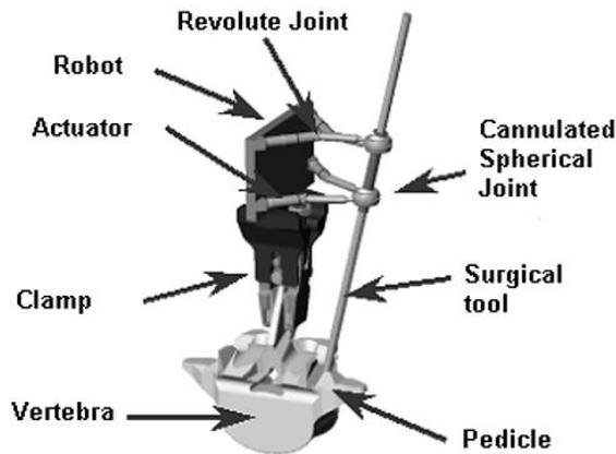
**Fig. 4.** A four DOF parallel bone-mounted robot. [10].
