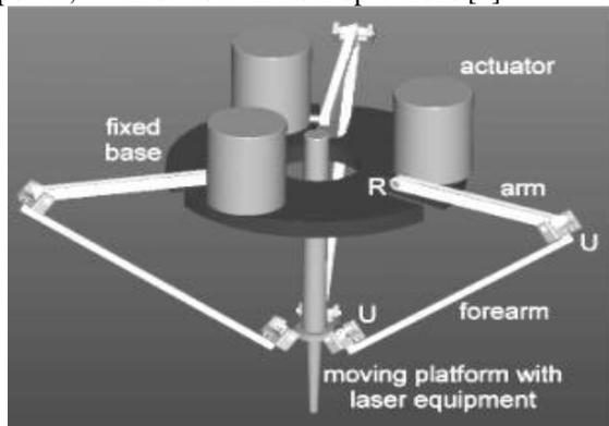
**Fig: 2.** parallel laser equipment [7].
