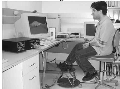
**Fig. 5.** The “Rutgers Ankle” Orthopaedic Rehabilitation System [12]
