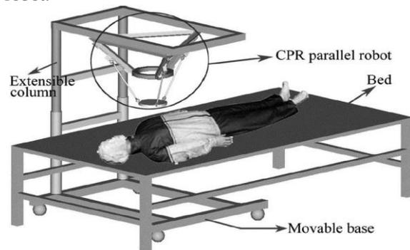
**Fig. 7.** Conceptual design of CPR operation [15].
