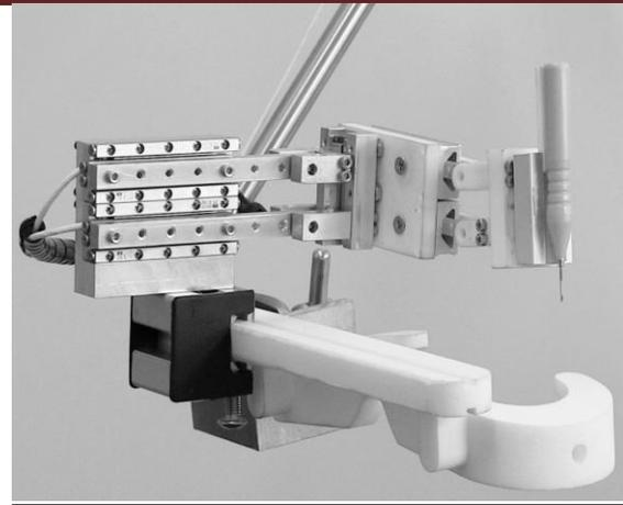
**Fig. 8.** 6DOF miniature robot designed for ophthalmic surgery
