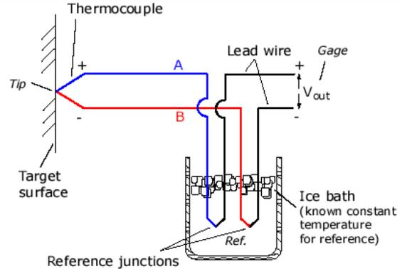
**Fig: 1.** Schematic Diagram for Calculation of Voltage Generated
