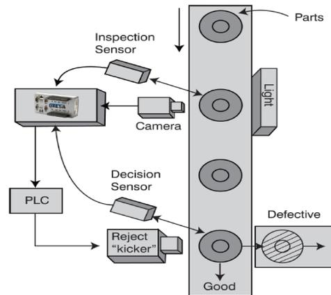
Fig. 1. Principle of Machine Vision System
