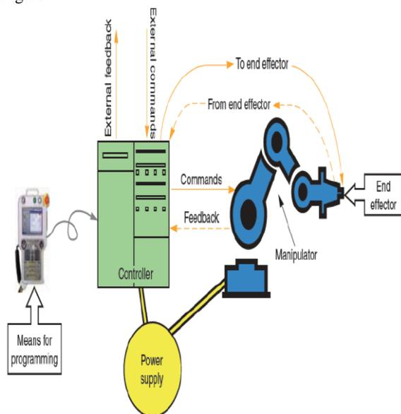
The controller is the part of a robot that coordinates all movements of the mechanical system. It also receives input from the immediate environment through various sensors. The heart of the robot's controller is generally a microprocessor linked to input/output and monitoring devices. The commands issued by the controller activate the
