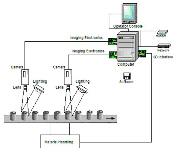
Fig. 2. Components of Online Machine Vision System
