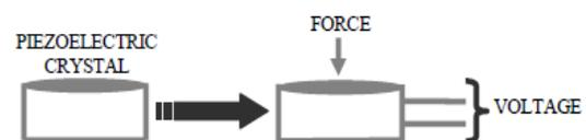
Fig. 1. Piezoelectric Effect
