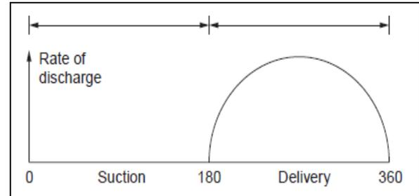
**Fig. 2.** Flow Variations during Crank Movement of Single Acting Pump
