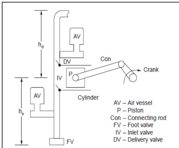
**Fig. 1.** Diagrammatic view of Single Acting Reciprocating Pump
