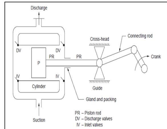
**Fig. 3.** Diagrammatic view of a Double Action Pump
