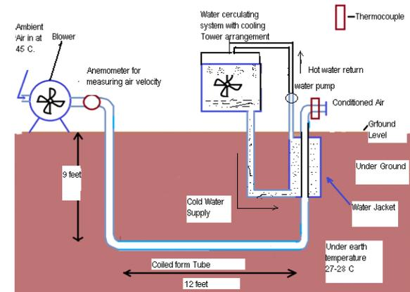
Fig. 1. Experimental set up of EAPHE
