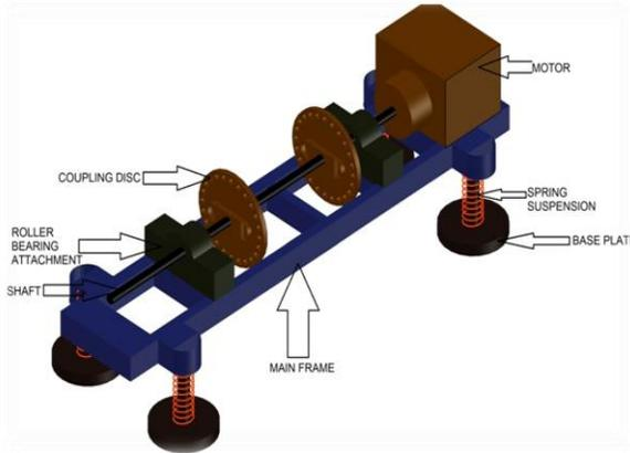
Fig: 1: CAD model of Experimental Setup. A Vibration Analyzer is attached on the roller bearing attachment on the free end of the Rotating Shaft
