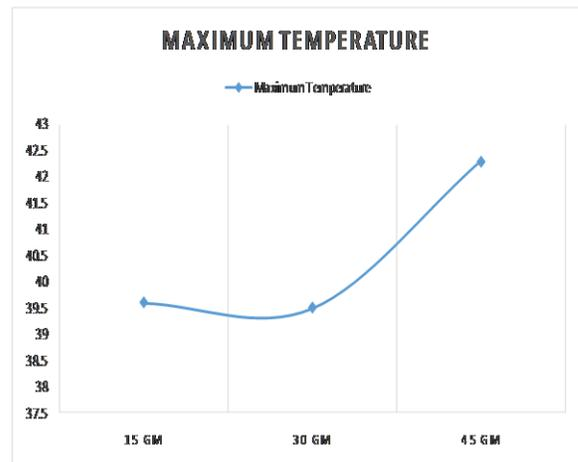
Fig: 3. Variation of Maximum Temperature with Weights under Mass Imbalance Condition
