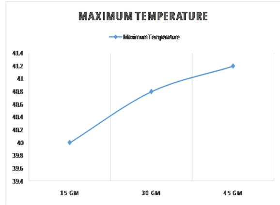
Fig: 2. Curve representing Variation of Maximum Temperature with Weights used for mass Imbalance with a ball bearing having ball Defect
