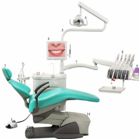
Fig. 1. Schematic Representation of a Dental Chair [3]
