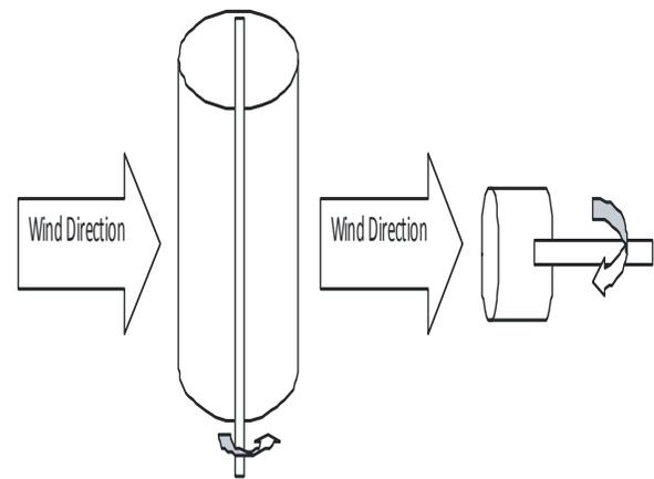
**Fig. 2.** Rotor Orientation [4]
