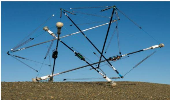
**Fig. 10.** “SuperBall” an Icosahedron Deployable Tensegrity Robot under Development in NASA [26]
