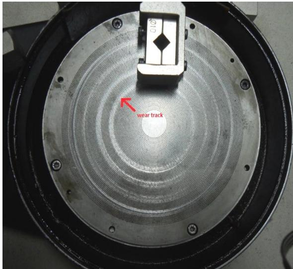
Fig: 10 Etched Mild Disc during Wear Test
