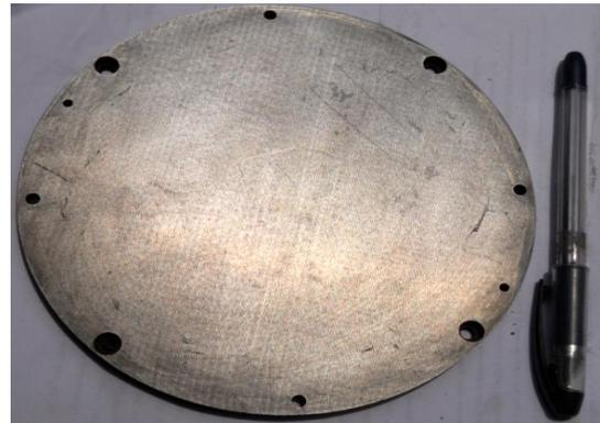
Fig: 5. Mild Steel Disc Before Etching
