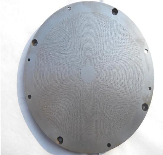
Fig: 9 Etched Mild Disc before Wear Test
