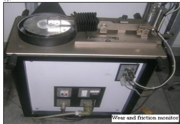
Fig: 8 Wear and Friction Monitor Machine for Pin on Disc Test
