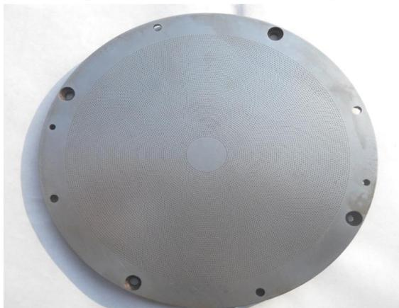
Fig: 7. Hexagonal Micro Holes on Disc by Chemical Etching
