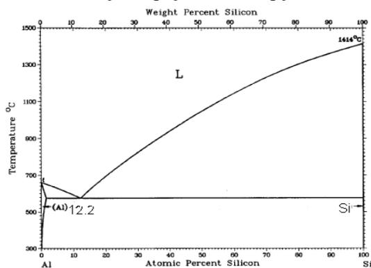
**Fig. 1.** Aluminium Silicon Binary Phase Diagram. The Eutectic Occurs at 12.6 wt% Si [3]
