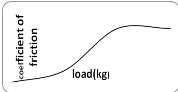
**Fig: 12.** Shows the Variation of Coefficient of Friction Vs. Load
