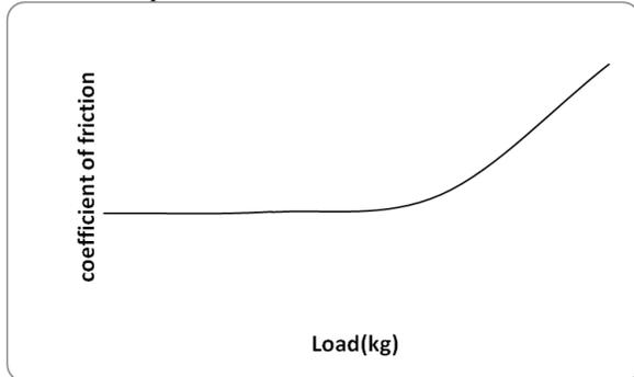
Fig. 9. Shows the Variation of Coefficient of Friction Vs. Load for Aluminum Alloy
