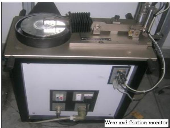
**Fig: 4.**Wear and Friction Monitor Used for the Wear Tests
