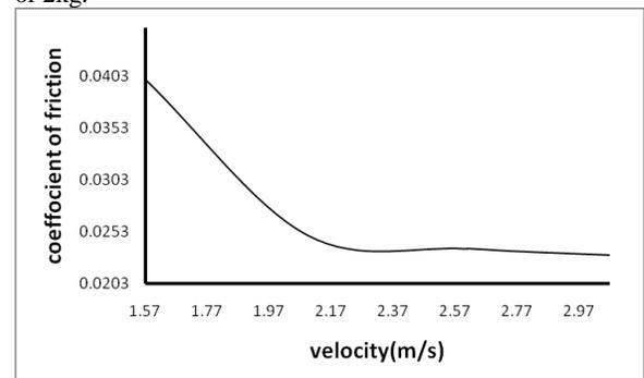
**Fig: 8.** Shows the Variation of Coefficient of Friction with Velocity for Aluminium Alloy
