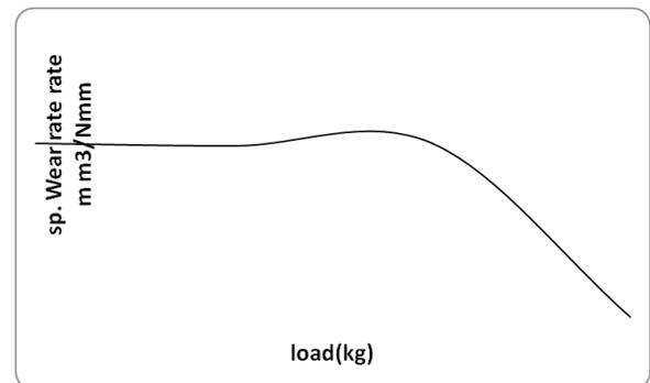
**Fig: 7.** Showing the Variation of Specific Wear Rate Vs. Load for Aluminium Alloy
