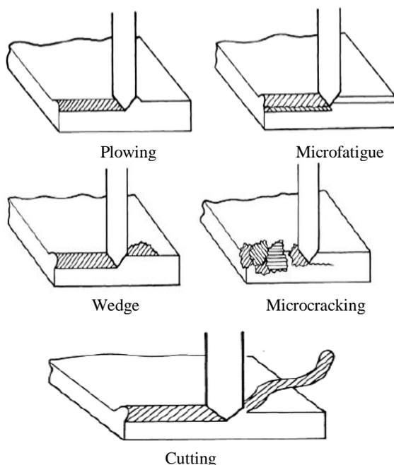
Fig. 2. Five processes of Abrasive Wear [4]
