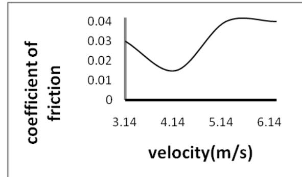
Fig: 11. Shows the Variation of Coefficient of Friction V.S. Velocity
