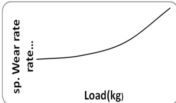
Fig: 10. Shows the Variation of Specific Wear Rate Vs. Load for Pure Aluminium
