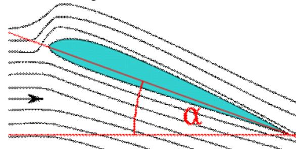
Fig: 5. Propeller Angle of Attack (alpha)
