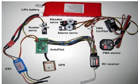
**Fig: 7.** General Schematic of the Electronics Components to be used
