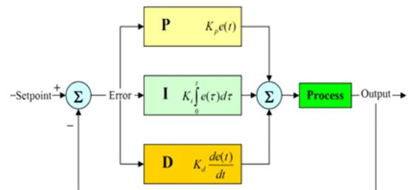
**Fig: 10.** Relevant STIMULINK Diagram to be applied for Quadrotor Control
