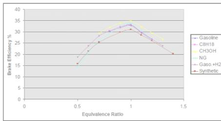
Fig. (1). Variation of brake efficiency with equivalence ratio for different fuels.
