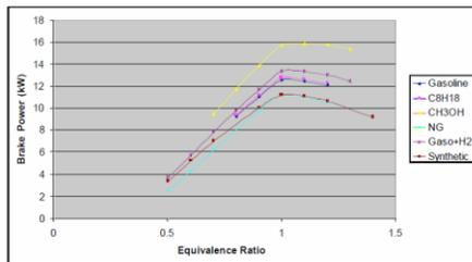
Fig. (2). Variation of brake power with equivalence ratio for different fuels.
