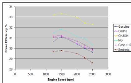
Fig. (3). Variation of brake efficiency with engine speed for different fuels.
