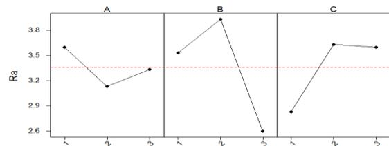
**Fig: 3.** Effect of Turning Parameters on Surface Roughness
