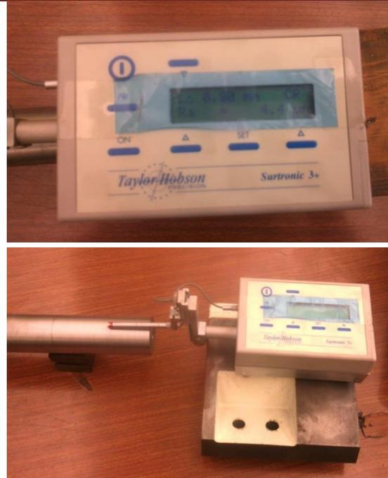
**Fig: 2.** Surtronic 3+, Roughness Testing Machine in Use
