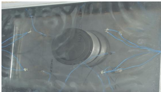
Fig. 3. Thermocouples Positions in Plate and Glass Covers
