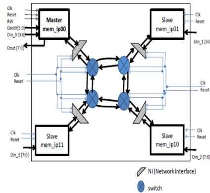
Top level block diagram for NOC architecture
