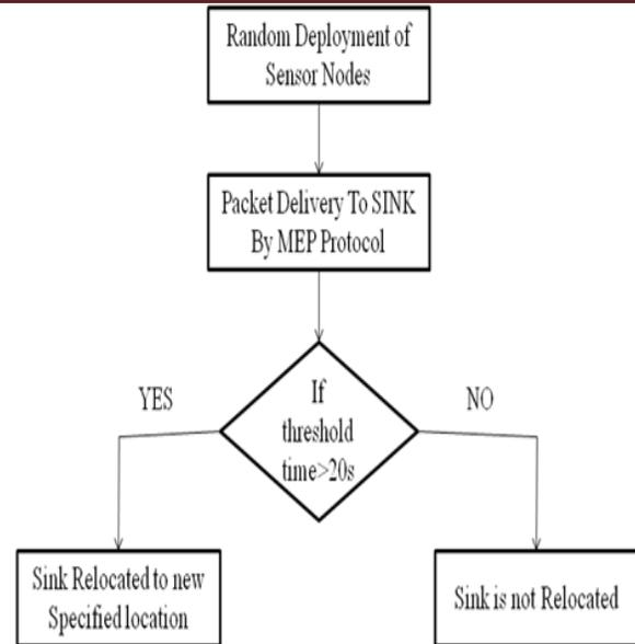
**Fig. 8.** Flowchart for Sink Relocation
