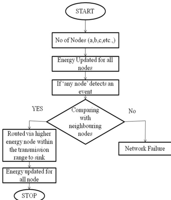
Fig. 5. MEP Operation Flowchart
