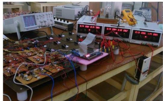
**Fig: 16.** Hardware Implementation of Single H Bridge MLI
