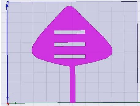
Fig. 1. Microstrip Snipped Patch Antenna
