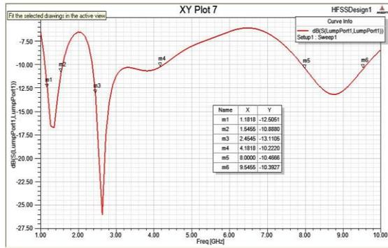
Fig. 2. Return Loss with Jeans Cotton as Substrate
