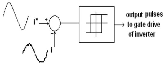
Fig. 3. Control Block Diagram for HBPWM
