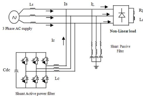
Figure 1. Hybrid Filter Configuration
