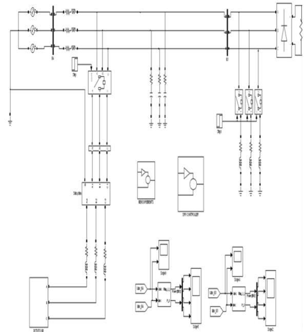
Fig. 4. Schematic diagram of SHPF with Hysteresis Controller
