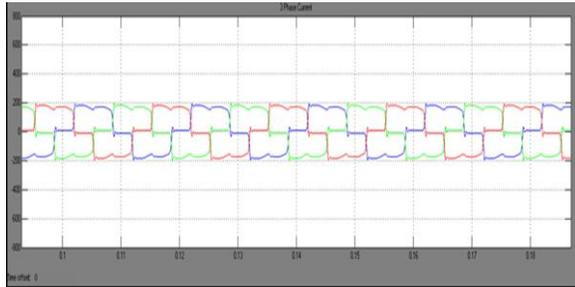
Fig. 6. Waveform of Supply Current (A) without filter
