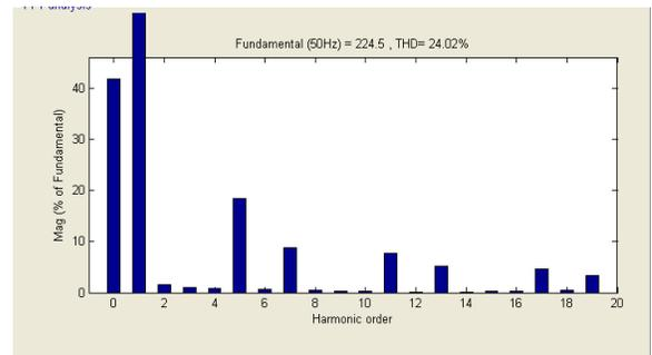
Fig. 12. THD calculation with HAP filter
