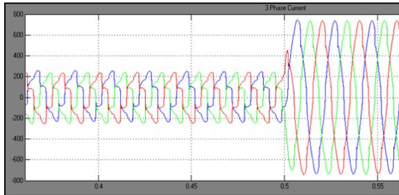
Fig. 8. Wave forms of HAP filter with hysteresis controller
