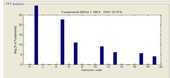
Fig. 11. THD calculation without filter
