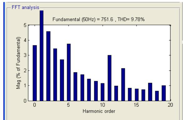
Fig. 13. THD calculation with HAP filter and hysteresis controller
