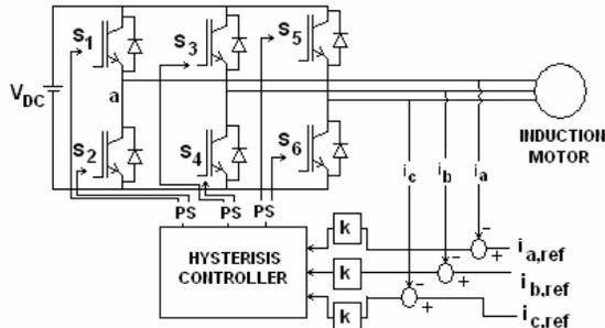
Fig. 2. Conventional HBPWM Inverter Control Method
