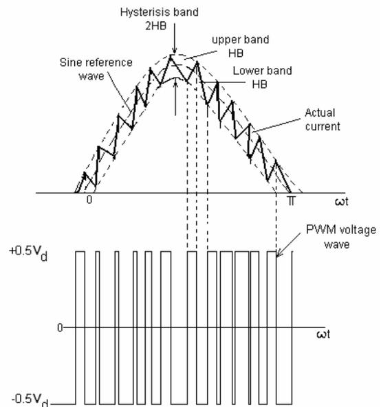
Fig. 1. Principle of Hysteresis Band Current Control
