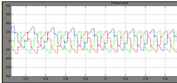
Fig. 7. Waveforms of Supply Current (A) with HAP filter
