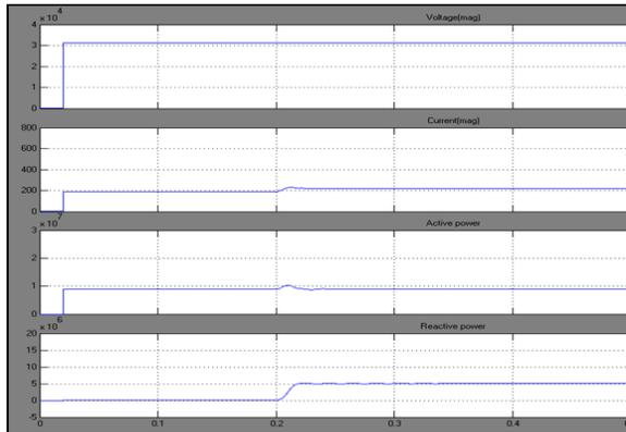
Fig. 9. Wave forms of (v), (A), reactive and real power before compensation
