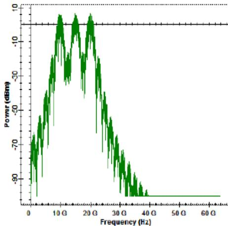
Fig. 2. RF Spectrums for Adding Three Channels at CS
