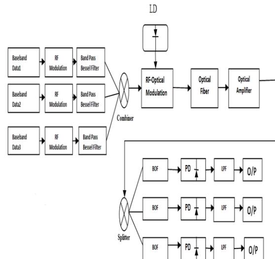
Fig. 1. Simulation Model of our Proposed SCM System
