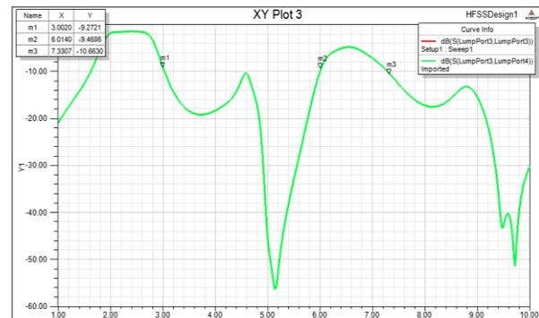
Fig. 5. HFSS plot of S11 and S21 versus frequency with the code giving the centre frequency as 3.75GHz for FR4 substrate for 0.5 dB ripple
