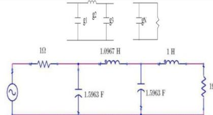
**Fig. 2:** A ladder network for a third order low pass Chebyshev filter prototype beginning with a shunt element.
