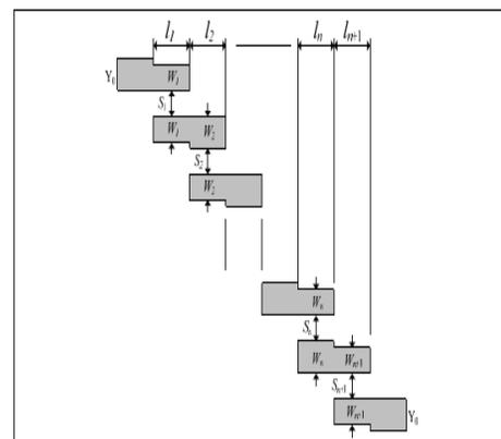
**Fig. 1.** General structure of parallel edge coupled strip line band pass filter
