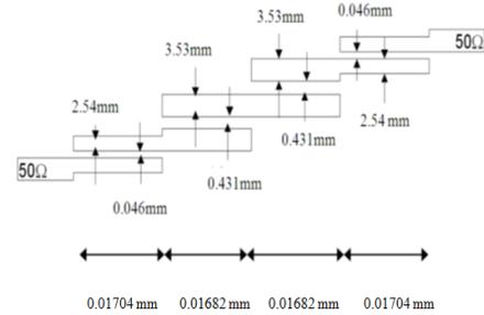
Figure 3: Layout of a three-pole micro strip edge-coupled band-pass filter
