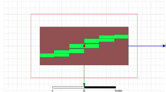
Fig. 4. Layout filter of 3rd order Edge couple Strip line band pass filter on HFSS
