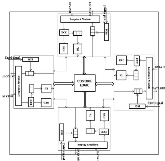
Fig. 2. Proposed Router Architecture
