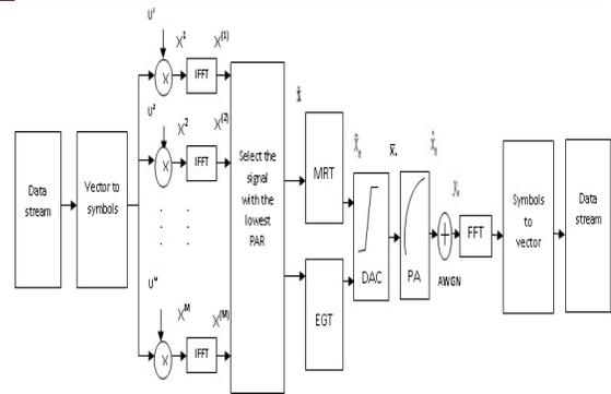
Fig. 1. PAPR reduction in MRT and EGT
