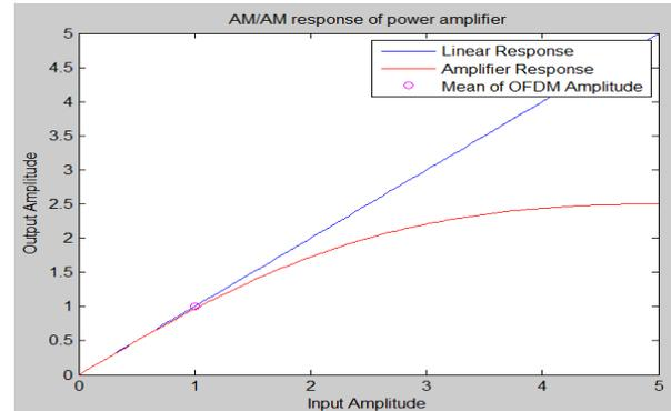
**Fig. 4.** AM/AM Response of Power Amplifier
