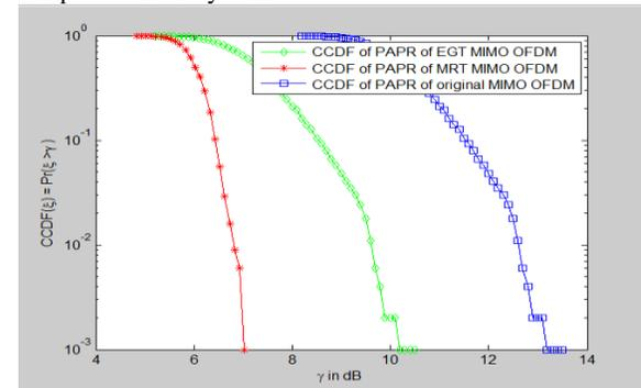
**Fig. 6.** CCDF of PAPR reduction for MRT and EGT system
