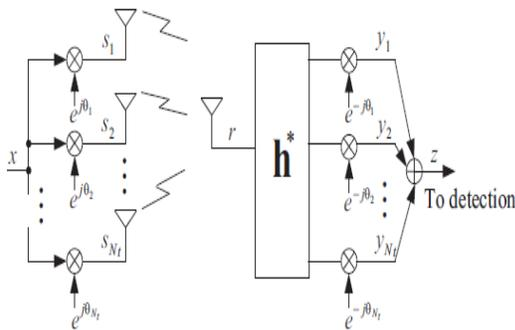
**Fig. 3.** Flow diagram of equal gain Pre-coder
