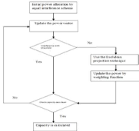
**Fig. 3.** Flowchart of the Proposed Gradient-Based Power Allocation Method
