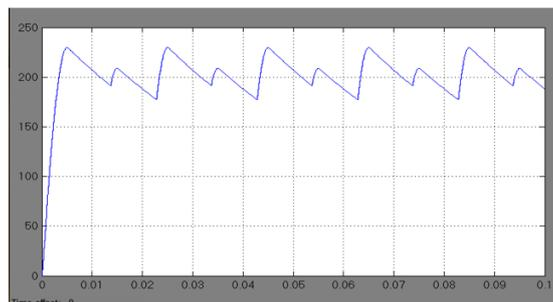
Figure 4 – DC grid voltage for Unidirectional ac to dc converter
