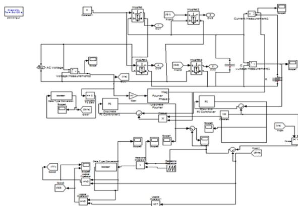
Figure 2 – Unidirectional ac to dc converter
