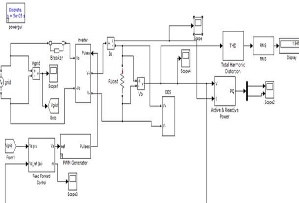
Figure 5 – Bidirectional ac to dc converter
