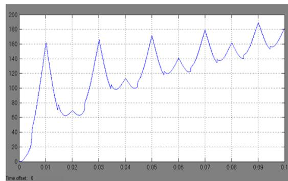
Figure 7 –DC grid voltage for bidirectional ac to dc converter
