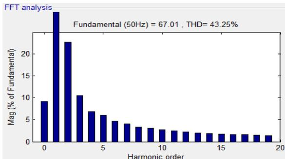
Fig: 16. THD Values for Output Voltage of DMC with RL Load
