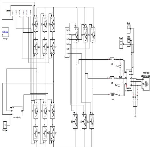
Fig: 8. Direct Matrix Converter Model for R Load
