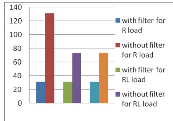
Fig. 24. Output Current of DMC for Various Load
