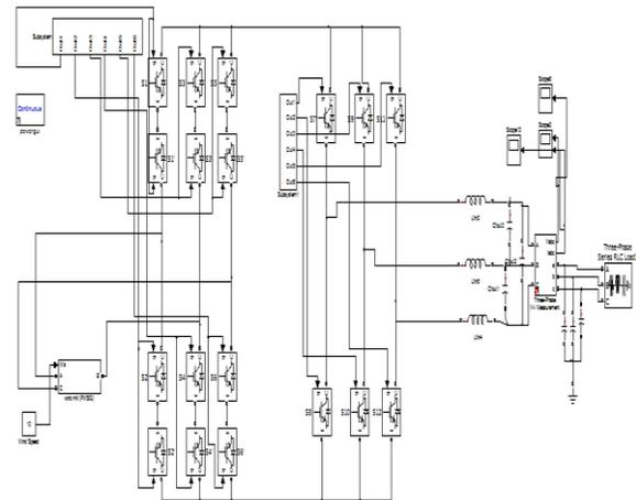
Fig: 18. Direct Matrix Converter Model for RLC Load
