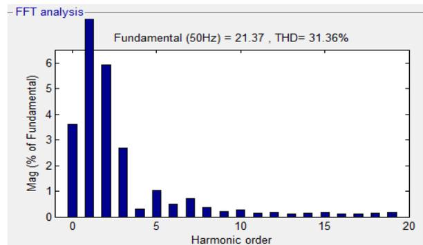
Fig: 12. THD Values for Output Current of DMC with R Load
