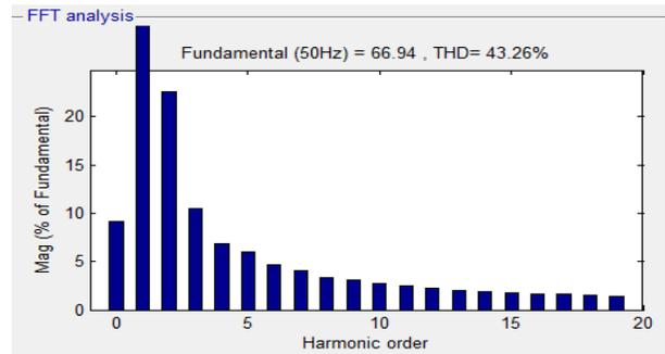
Fig: 11. THD Values for Output Voltage of DMC with R Load
