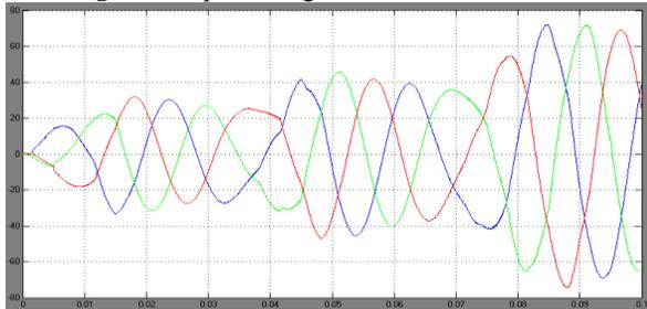
Fig. 20. Output Current of DMC for RLC Load
