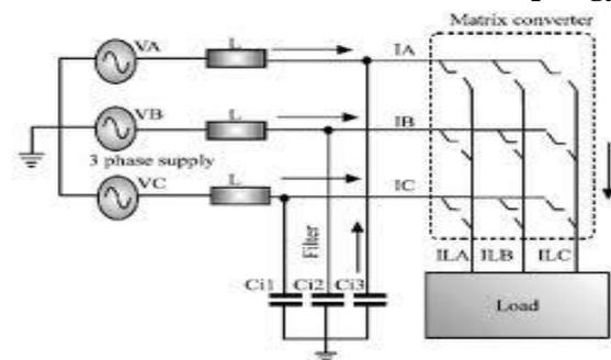
Fig. 1. Three Phase Matrix Converter
