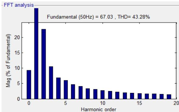
Fig. 21. THD Values for Output Voltage of DMC with RLC Load
