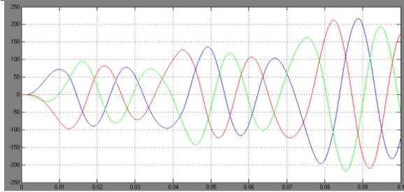
Fig. 19. Output Voltage of DMC for RLC Load
