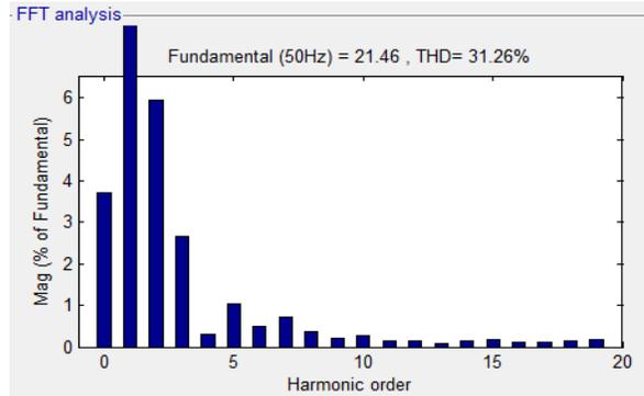
Fig: 17. THD Values for Output Current of DMC with RL Load
