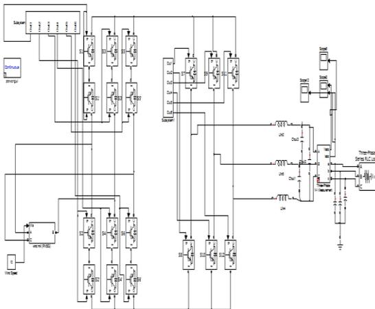
Fig: 2. Proposed Matrix Converter
