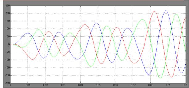
Fig: 9. Output voltage of DMC for R Load
