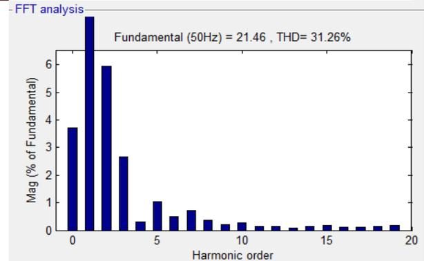
Fig. 22. THD Values for Output Current of DMC with RLC Load
