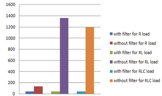
Fig. 23. Output Voltage of DMC for Various Loads
