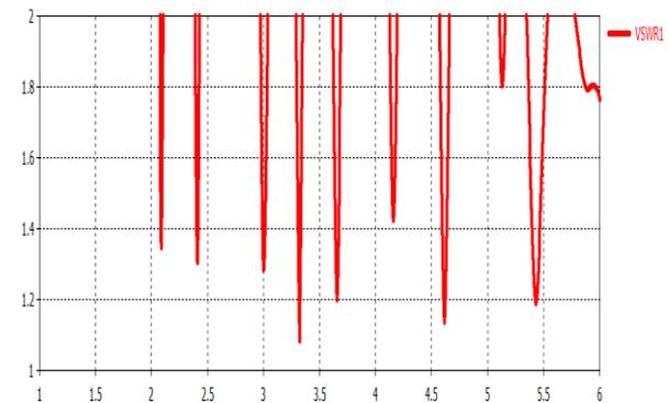
**Fig. 5.** VSWR plot of the multi band patch antenna with H and U slots
