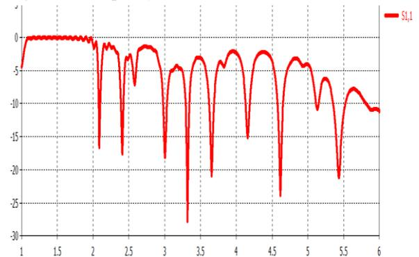
**Fig. 4.** Return loss of the Multi Band Patch Antenna with H and U slot
