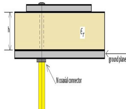
Fig. 1. Geometry of the Coaxial fed Microstrip Patch Antenna
