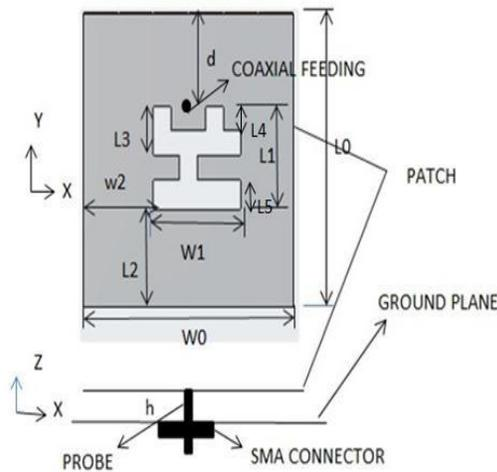
**Fig. 3.** Geometry of the Multiband Microstrip patch antenna with H and U slot (Top view)
