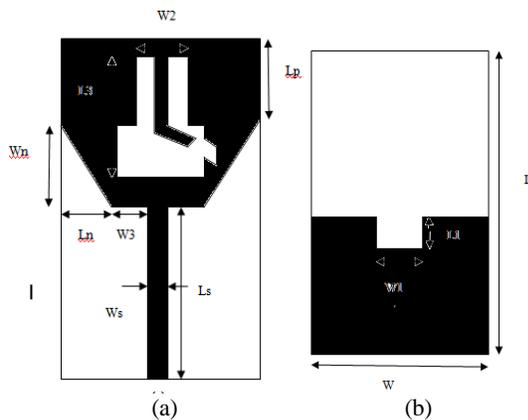
**Fig. 1.** Configuration of the proposed compact slotted patch antenna for wideband application: (a) top view; (b) bottom view
