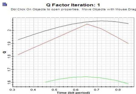
Fig: 7. Q-factor for Complementary Subtraction Method
