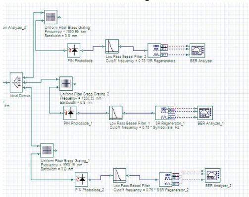
**Fig. 2. Direct Detection Technique**
