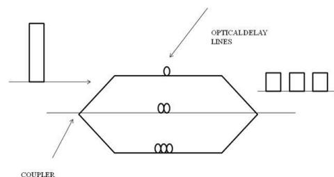
Fig: 1. Optical Delay Line Encoder
