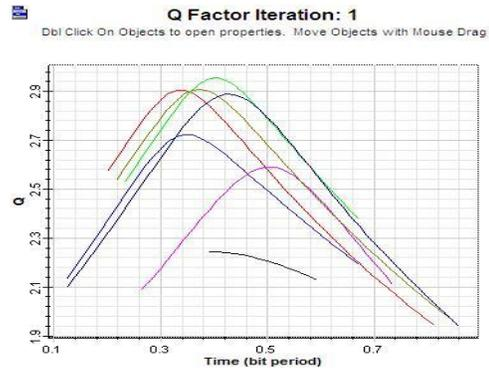
Fig: 8. Q-factor for Single Photodiode Detection
