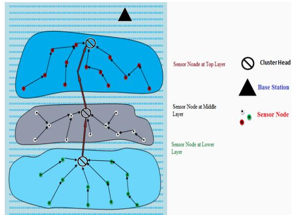
Fig. 4. Layer to Layer Transmissions
