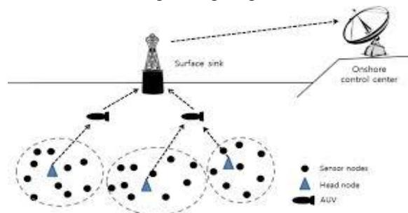
Fig: 1. Under Water WSN Architecture
